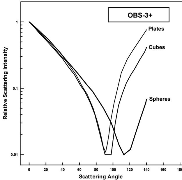
FIGURE 11-3. Relative scattering intensities of grain shapes
